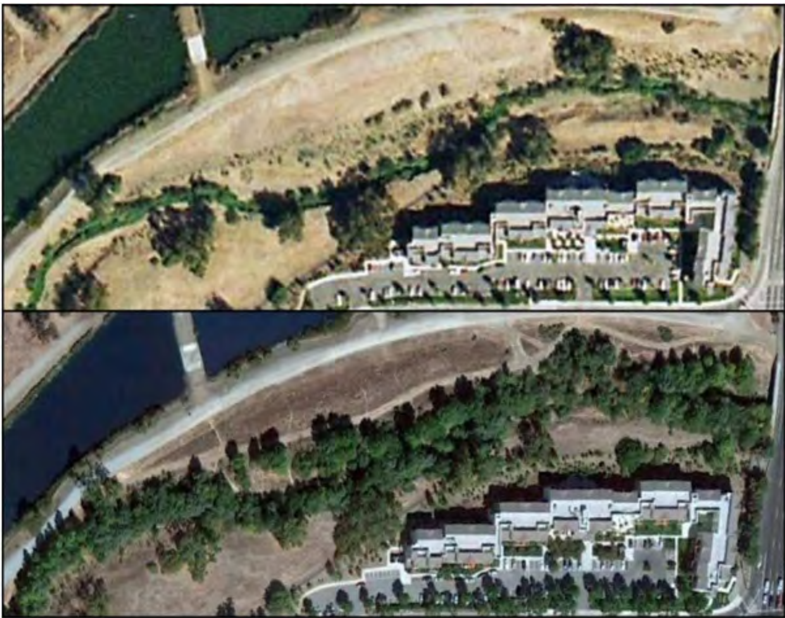
Figure 17. Example of Overexcavation on Guadalupe Creek to Enhance Subsurface Water Storage (top photo, before; bottom photo, after)
